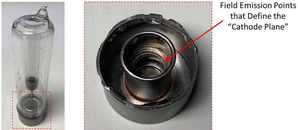
Fig. 18 Cathode cup removed from an L3 150-kV X-ray tube. The geometry shields the ability to inject magnetic field into the region where the anode interacts with the cathode plane.
