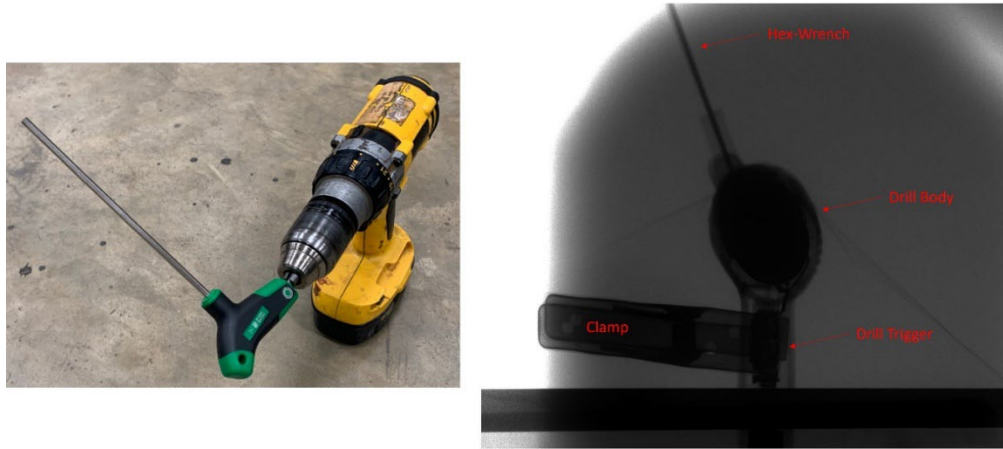
Fig. 13 Radiographic target (drill with a bent hex-wrench) and radiographic image from experiment 34 in which two electrical pulses were supplied to the X-ray sequencer 180 \mu s apart.
