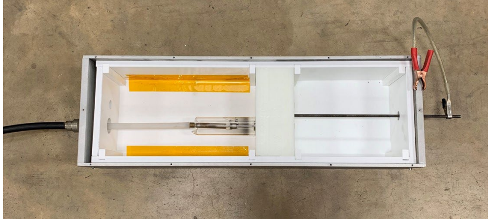
Fig. 16 Hardware to allow observation of plasma within off-the-shelf field emission X-ray tubes. Pulser (aside to the left).
