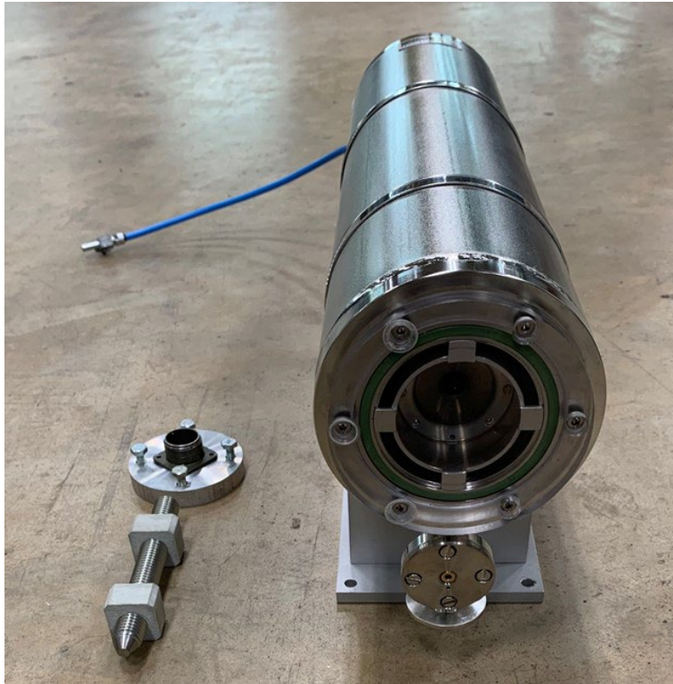
Fig. 21 Modifications of a Scandiflash XT 300L tube to include a transparent front cover and adapters to fit to an L3 150-kV pulser
