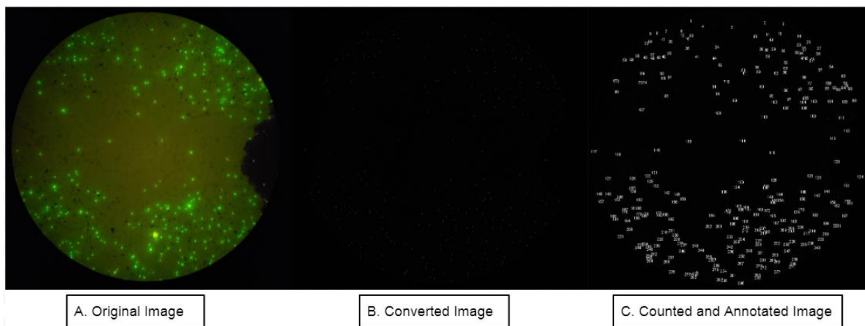
Figure 20: Steps in the Image-J Software Particle Counting Process, from Original Image (A), Converted into usable format (B), and Counted (C)
