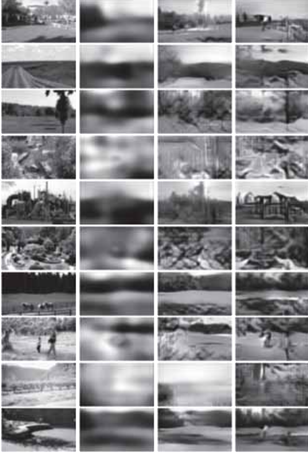
Figure 2. Reconstructed images with models using various loss terms. From left to right: original image, reconstruction with pixel loss, reconstruction with pixel and adversarial loss, reconstruction with pixel, feature and adversarial loss.
