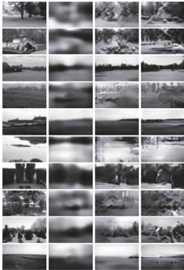
Figure 12. More reconstructed images with models using various loss terms. From left to right: original image, reconstruction with pixel loss, reconstruction with pixel and adversarial loss, reconstruction with pixel, feature and adversarial loss.
