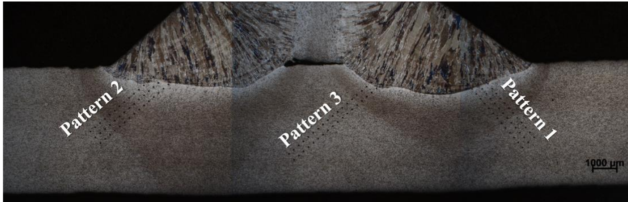
Figure 17. Composite image of light optical micrographs of the HSLA-80 fillet weld showing placement of microhardness indents. Indents appear as sets of parallel lines of black dots on the left, center, and right sides of the image.
