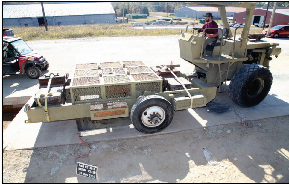
Figure 17. Aircraft load cart trafficking of repair craters.
