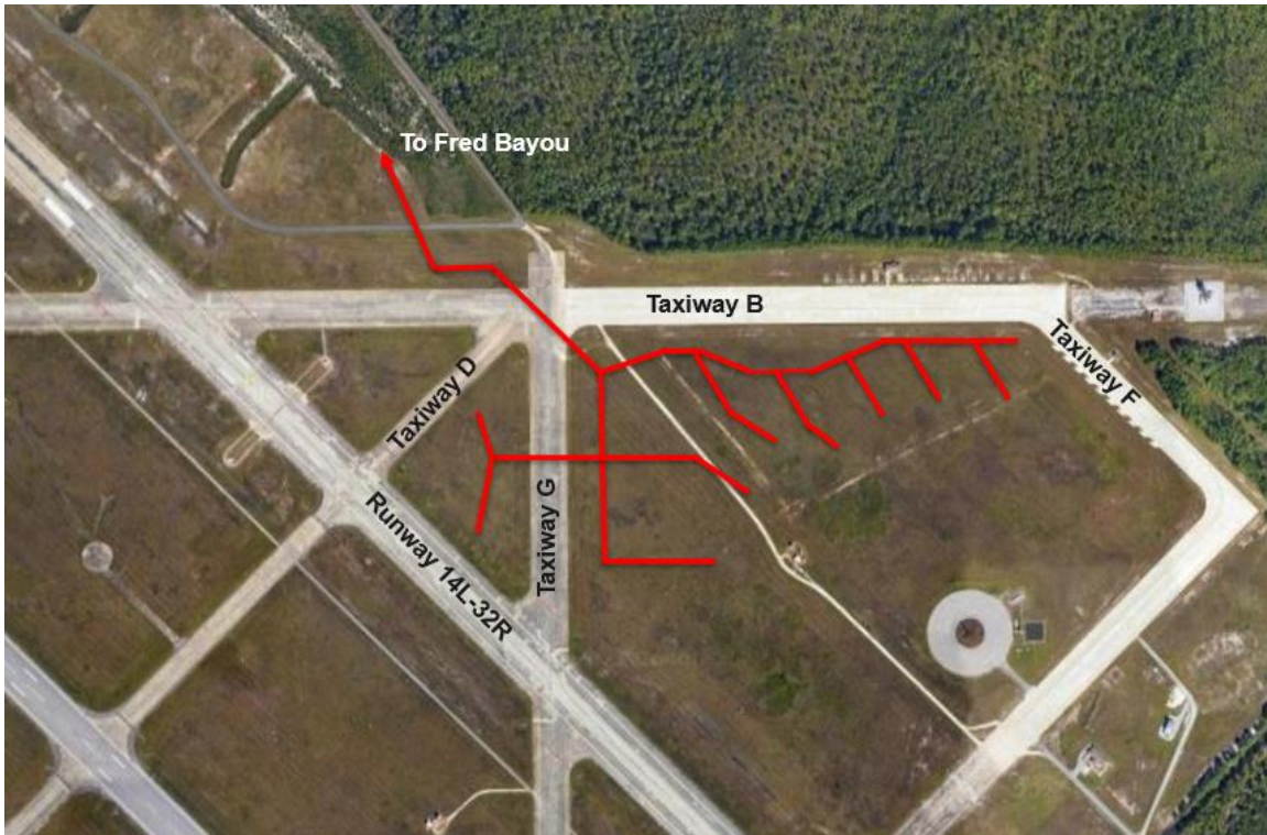
Figure 7: Modeled Stormwater System
