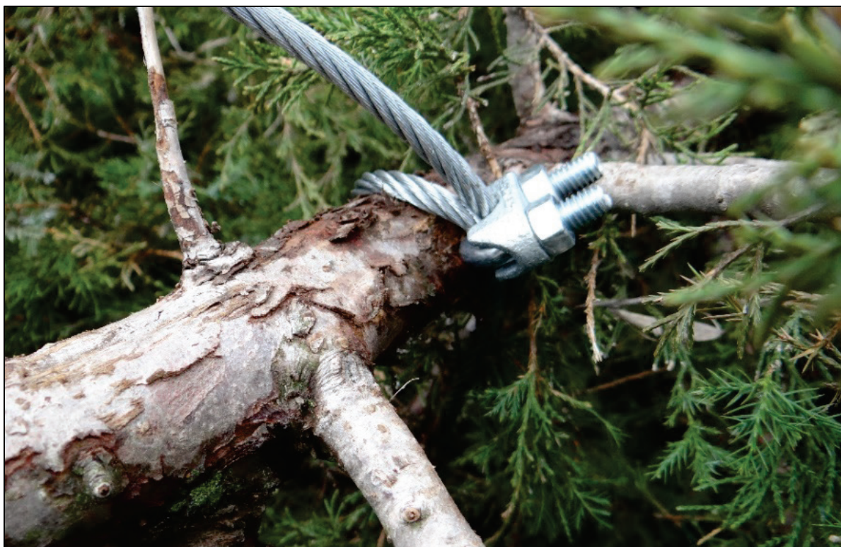
Figure 5. A cable clamp is used to secure the cable on the tapered end of a cedar tree. The coordinates for these connections are labeled “anchor points” in Table 1.
