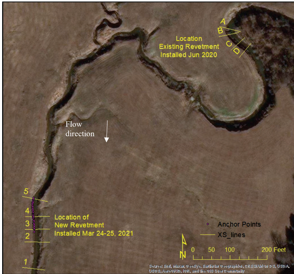
Figure 6. The locations of the cross sections collected at McConnell Creek. Five cross sections were collected at the downstream site, and four were collected at the upstream site. Upstream cross sections are labeled A through D while downstream cross sections are labeled 1 through 5.
