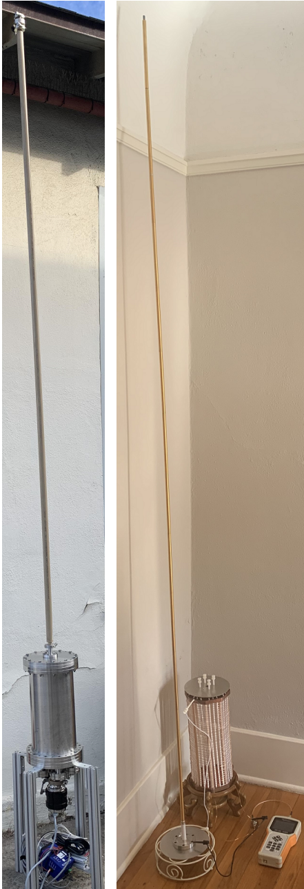
Fig. 2. The left photo shows the cryogenic system, and the right photo shows the antenna and tuner designed to be installed within this cryogenic system.
