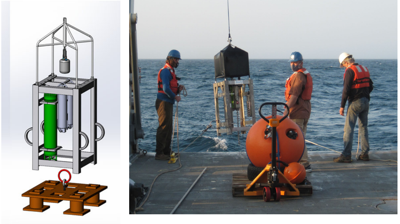
Fig. 4 (Left) IVAR-2 system showing sensor within the protective upper frame; below this are data acquisition system (green) and expendable anchor that is released on recovery. (Right) IVAR-2 being recovered from the R/V Armstrong by David Dall'Osto (left), Eric Boget (right) and R/V Armstrong crewmember (center). A shroud (spandex-like material) covers the frame and sensor and provides a highly effective reduction in bottom currents which can result in flow noise and sensor motion that degrades measurement. The large buoy (31-inch diameter) seen in foreground floats 7 m above IVAR-2 and provides necessary flotation for recovery.
