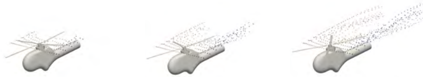
Fig. 8 In situ particle path and surface extract outputs for Higher-harmonic control Aeroacoustics Rotor Test II case. Images used with permission from Andrew Bauer courtesy of Kitware Source Quarterly Magazine.
