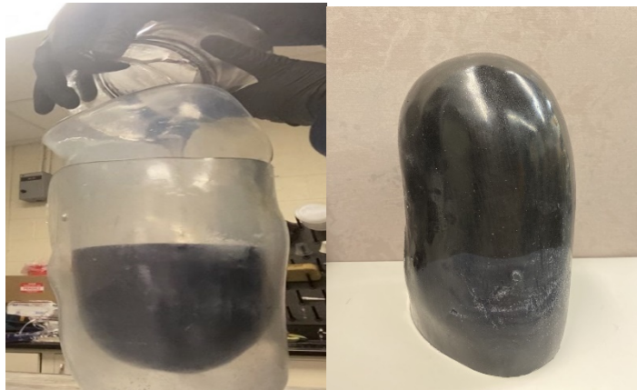
Figure 9 (Left) Pouring liquid silicone rubber into the socket to fabricate another plug for laboratory testing, and (Right) Fully cured silicone plug
