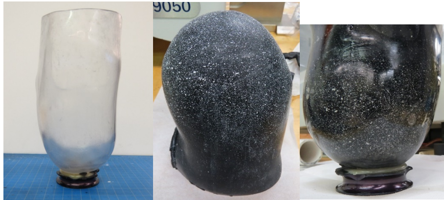
Figure 1 (Left) Diagnostic socket, (Middle) Black silicone plug with white acrylic paint speckle pattern, (Right) Plug inserted into diagnostic socket
