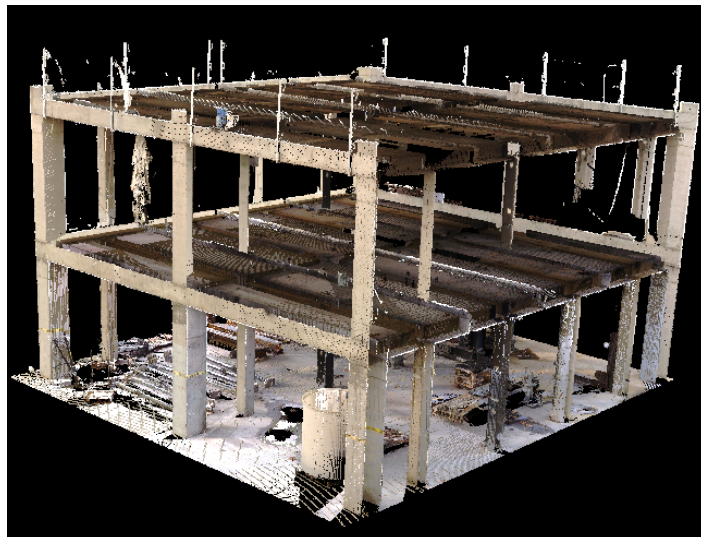
Figure 8: Original point cloud of seismic testing structure
