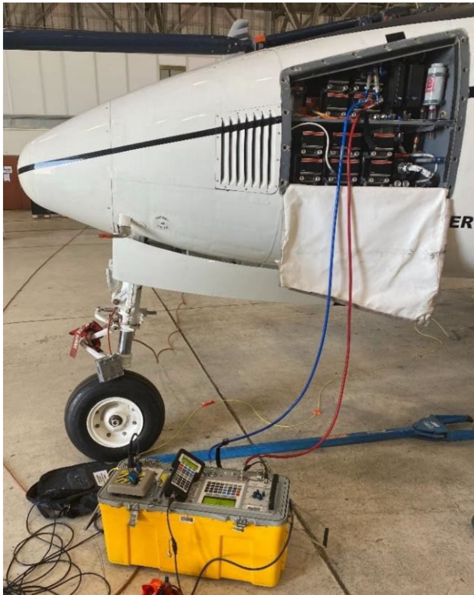
Figure A2. Druck™ ADTS 405 Connected to ADC 1
