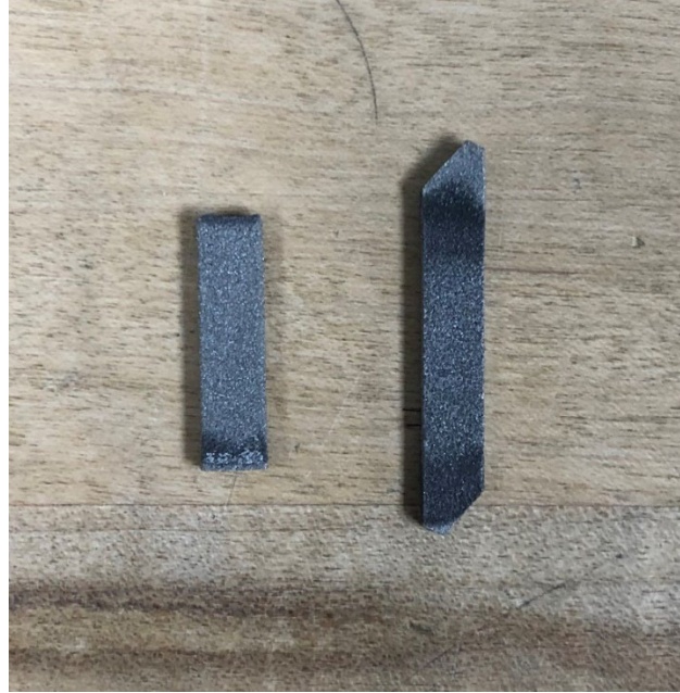
Figure 3.2 Printed 70% Mo 25% W 5% Re vertical sample (left) and 45° sample (right)
