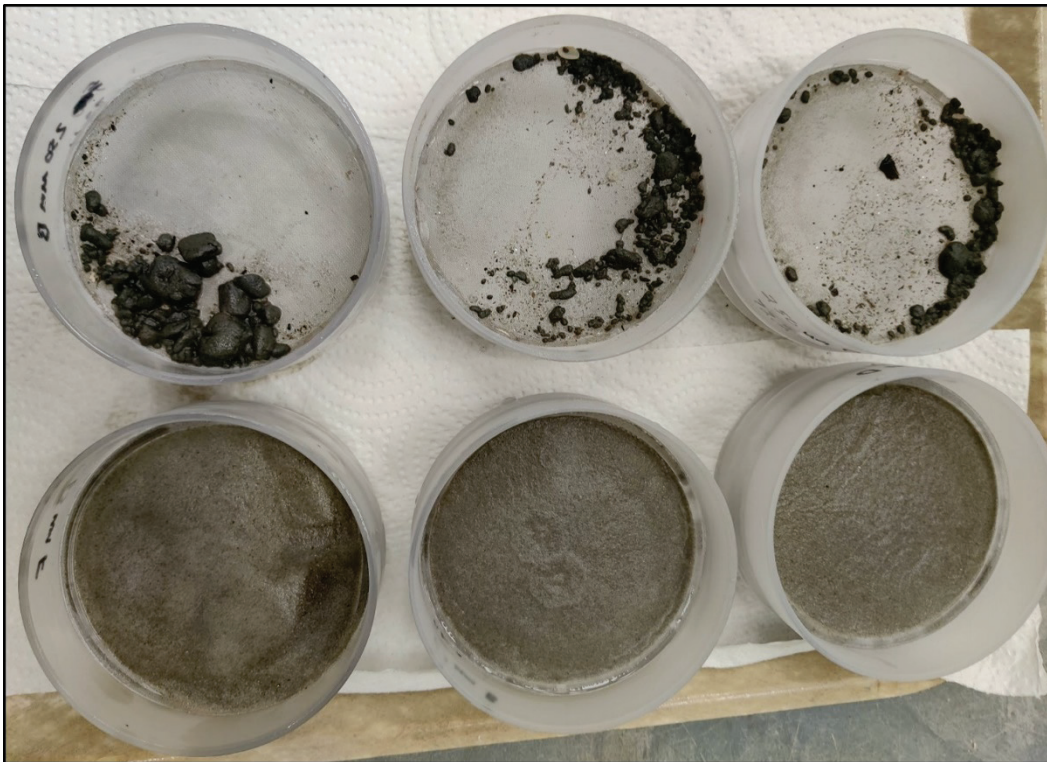
Figure 11. Photographs of Cumberland Sound RG sediment retained on 250 \mu\text{m} sieves (top) and 63 \mu\text{m} sieves (bottom).
