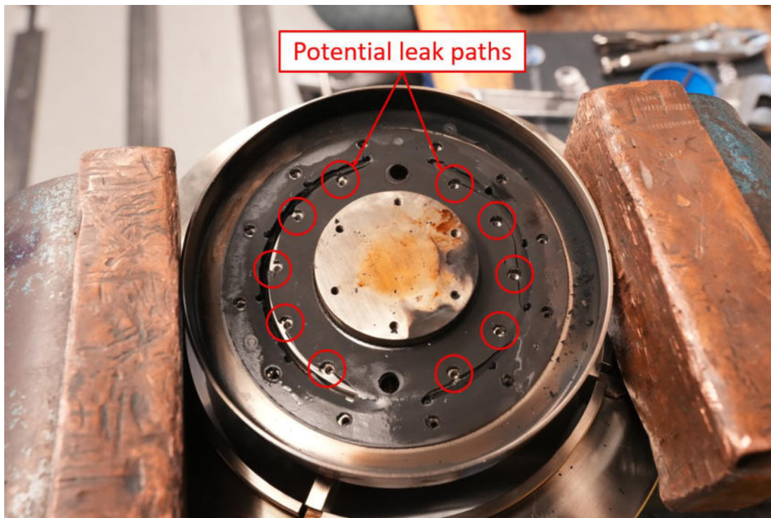
Figure 141. Fuel manifold gasket after the third iteration of testing
