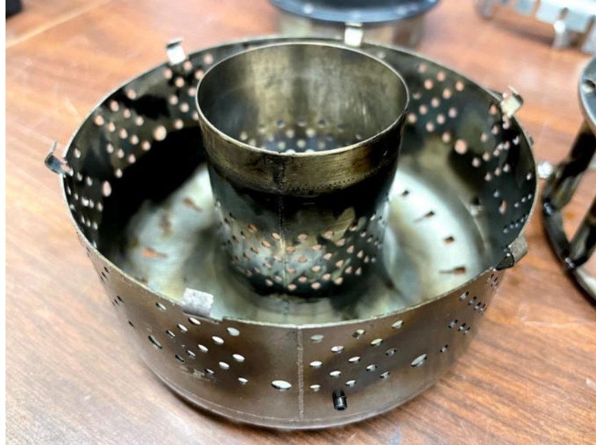
Figure 42. P160 compact combustor outer and inner liner mated to the forward dome after machining and laser-welding
