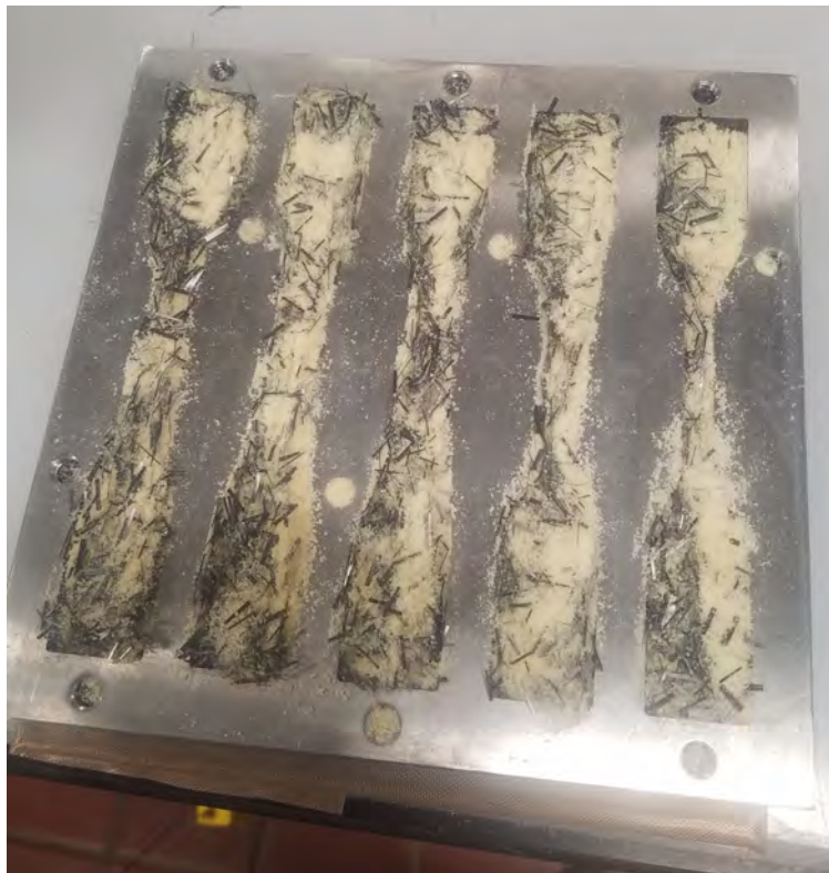
Figure 73. ULTEM 1000-carbon fiber within 3-piece Compression Mold
