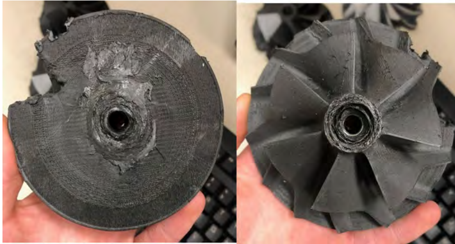
Figure 52. Murphy 1st onyx CF compressor [89]
