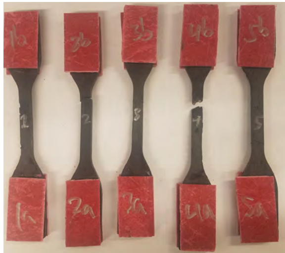
Figure 116. Epoxy-CF Specimens Batch 6 (10% reinforcement)
