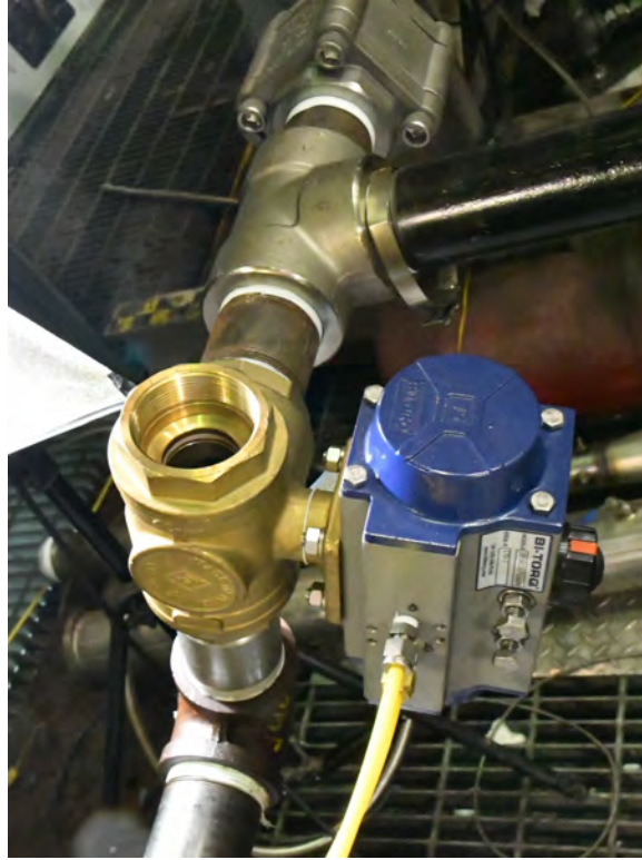
Figure 92. Safety Feature on Test Stand: Pneumatic Three-Way Globe Valve.
