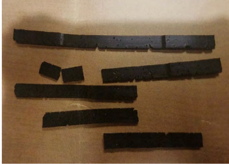
Figure 61. Batch 1: Traditional Dogbone Shape
