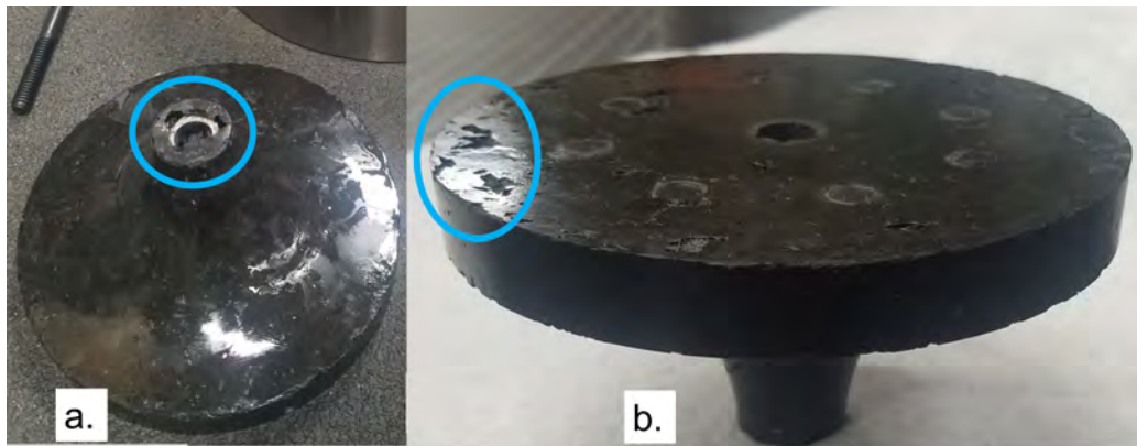
Figure 153. Epoxy-Carbon Fiber Surface Finish
