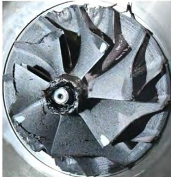
Figure 51. Carbon fiber onyx compressor failure [1]
