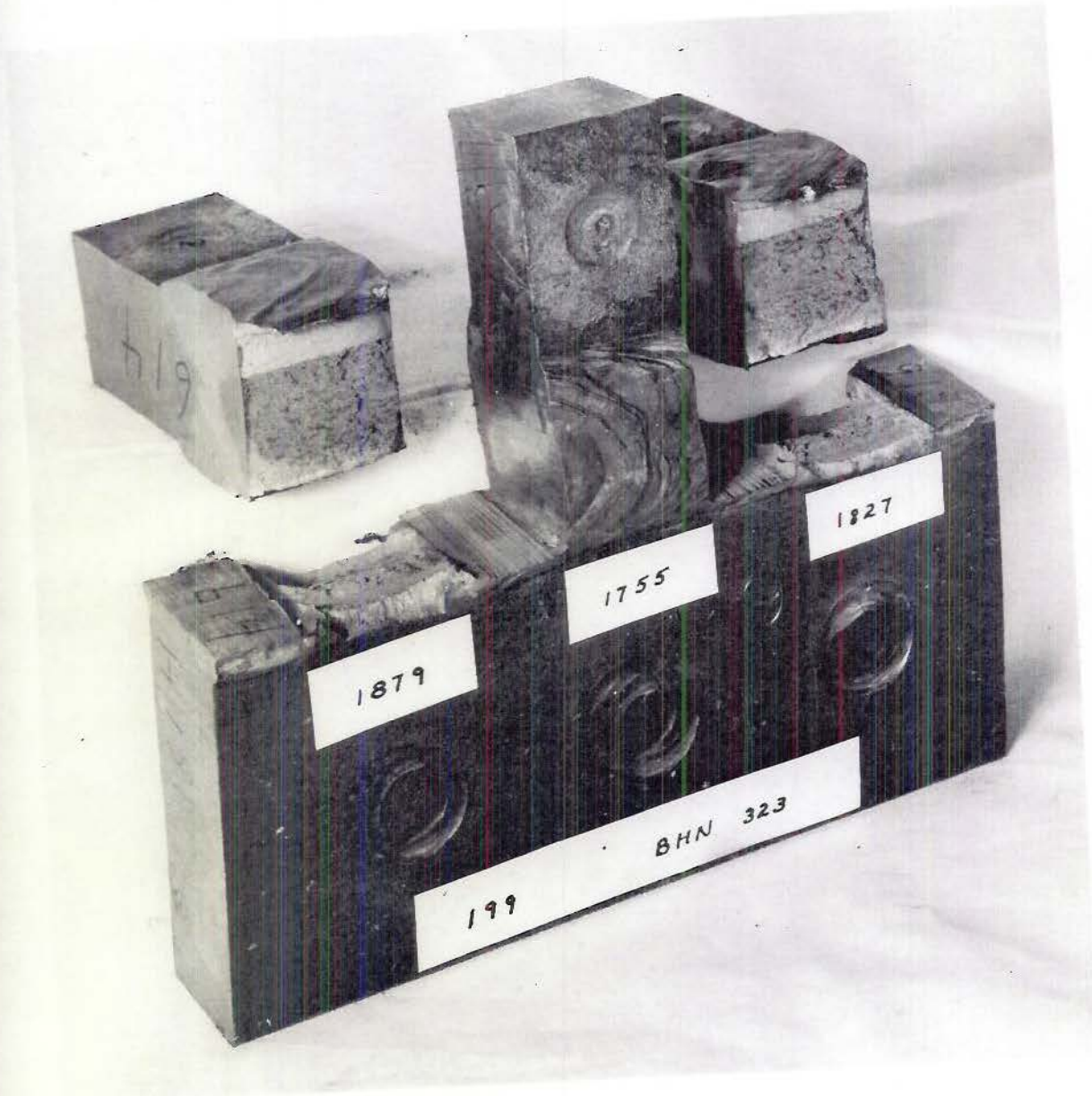
NRL SHOCK FRACTURE SPECIMEN. DOUBLE V WELDS AT BASE OF FINGERS.
