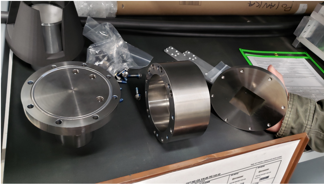
Figure 27. Base (L), Cryogenic Cavity (C), Dry Ice Holder (R)
