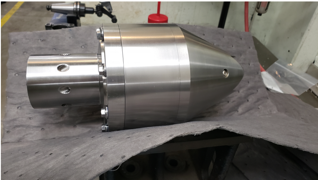
Figure 28. Fully Constructed Dry Ice Holder
