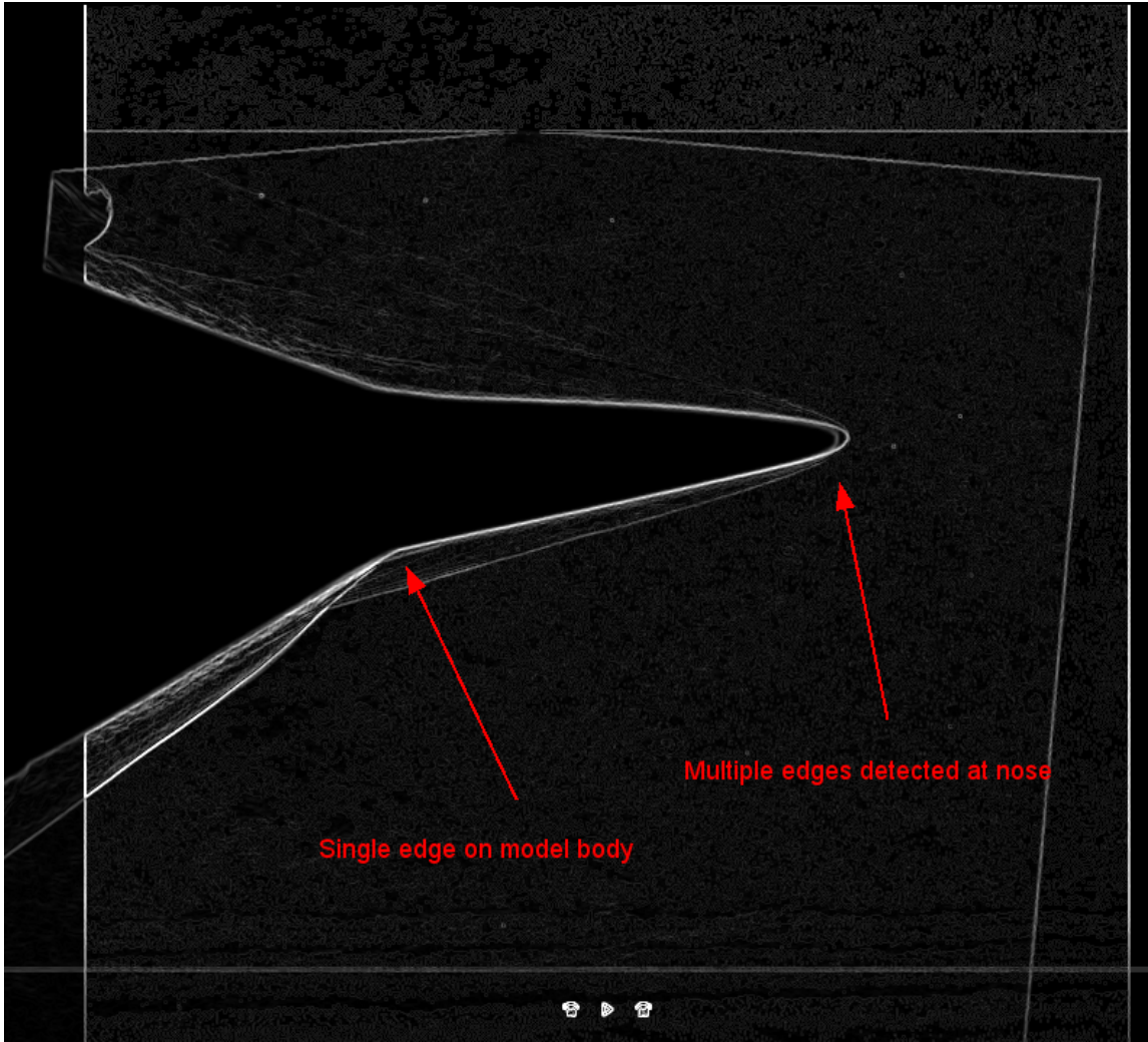
Figure 52. Overlaid Bi-conic Images Showing a Single Body Edge and Multiple Nose Edges
