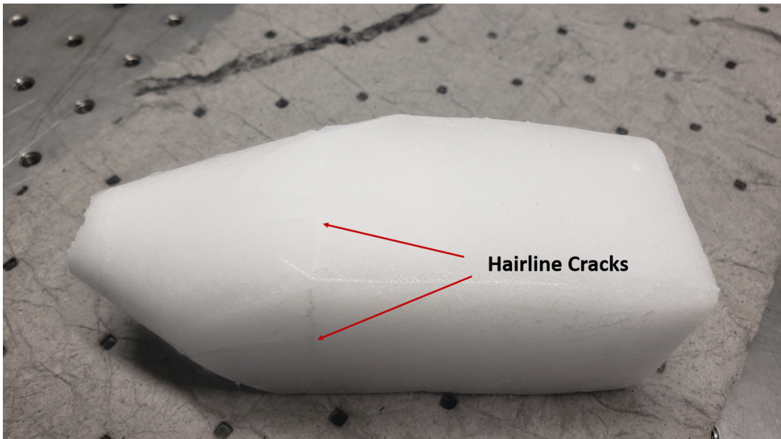
Figure 19. Ice Model with Hairline Cracks
