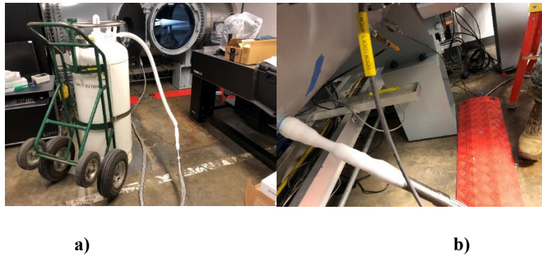
Figure 15: Post Run 44, a) Cryogenic Dewar Attached to Cryogenic Hose system, b) Transfer Line Connector into the Tunnel Test Section
