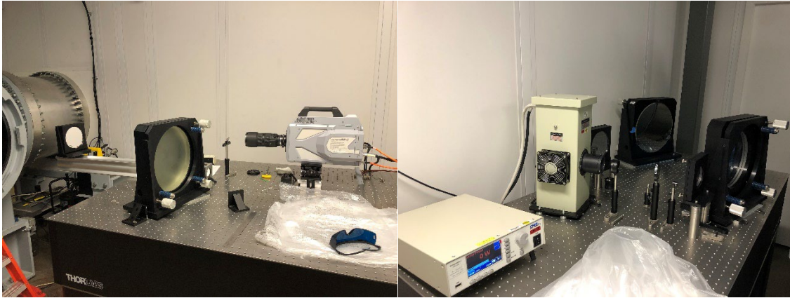
Figure 21: Physical Schlieren set-up for experiments
