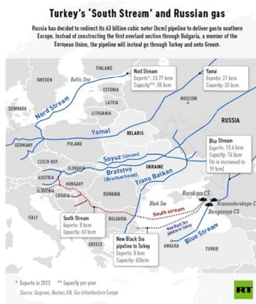
Figure 2: Russia-Europe gas pipelines 4
