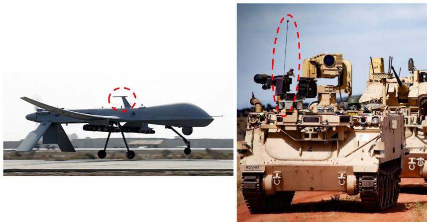
Figure 10: Both the blade antenna on an MQ-9 (left) and the whip antenna on a Bradley (right) are good candidates for replacement by MDWAs and MFCs.
