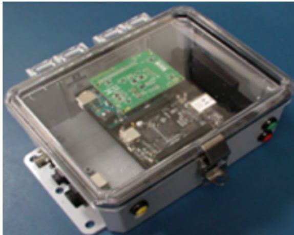
Figure 18. The Merlyn multimodal detection platform measures multi-phenomenological signals simultaneously at a 16 Hz sampling rate [81].
