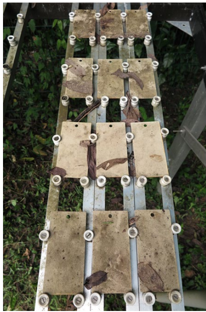
Fig. 6 MIL-DTL-64159B (2015) full rack of panels after 18 months' outdoor exposure in Afobaka, Suriname
