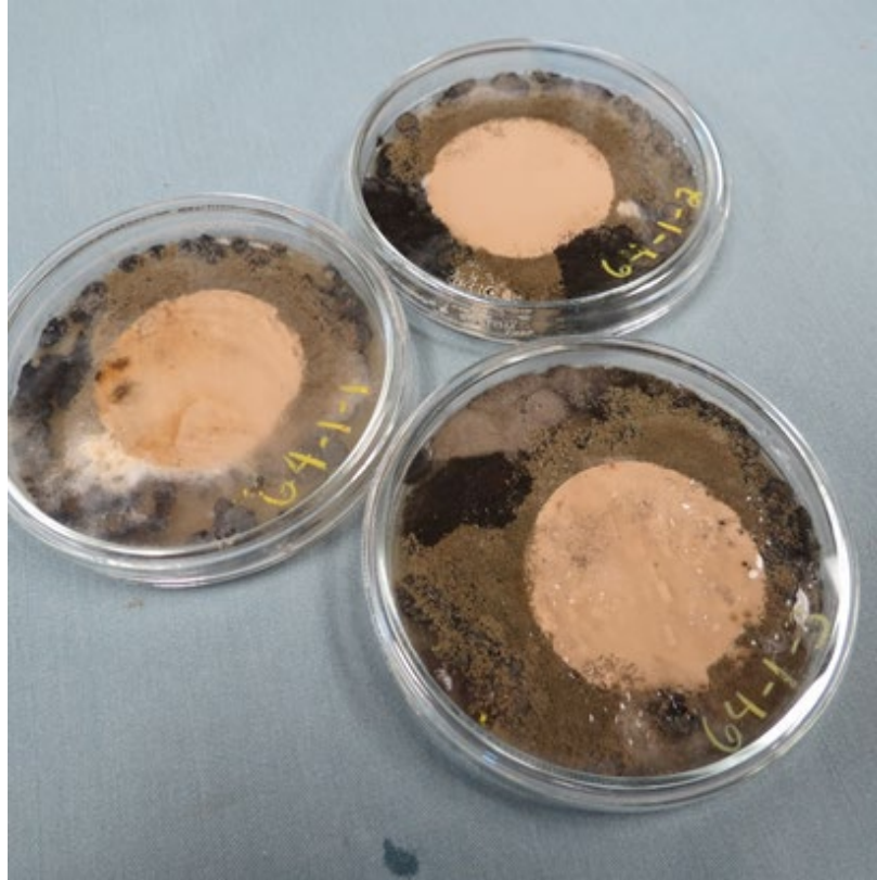
Fig. 1 MIL-DTL-64159B (2015) control coatings (without biocide additive). Trace to light growth was observed, ASTM D5590 (2017) (Aberdeen Test Center [2019]).
