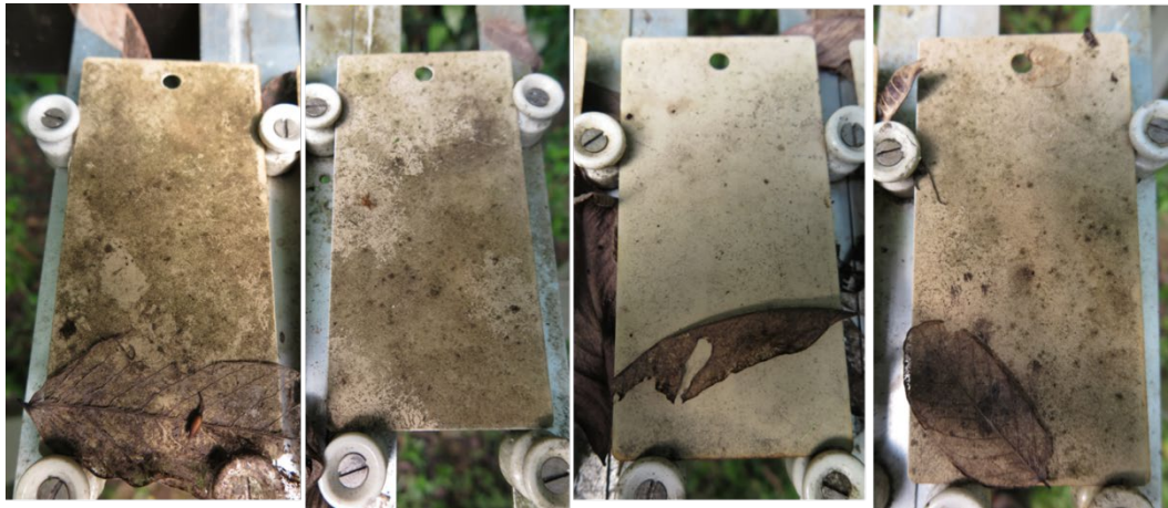
Fig. 7 MIL-DTL-64159B (2015) panels after 18 months' exposure in Afobaka, Suriname. (Left to right) Control 0% ZPT, 0.15% active ZPT, 1.11% active ZPT, 0.11% active ZPT/0.285% IPBC blend.
