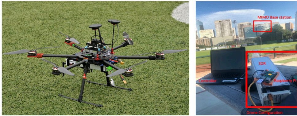
Fig. 2 Drone and controller: (left) drone equipped with sensors, battery, and antennas ready for take-off; (right) controller setup where we see the massive MIMO base station on top of a building, the software-defined radio (SDR)-Pi configuration that will be connected to the drone, and a computer as a controller
