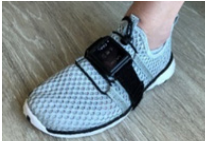
Figure 1. Inertial sensor (Opal) placement on the foot dorsum.
