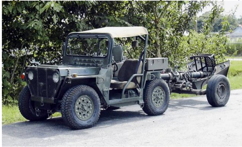
Figure 6. 120mm Expeditionary Fire Support System (EFSS) w/ Internally Transportable Vehicle (ITV)
