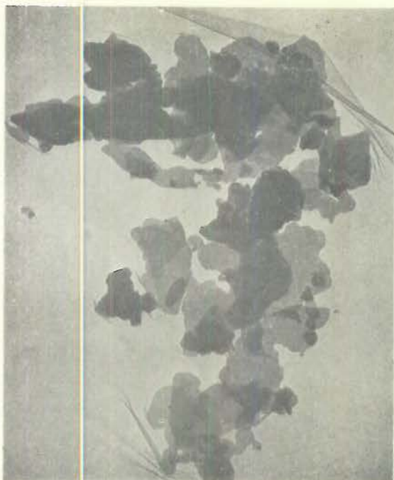
A AN ARSENIC INSECTICIDE SHOWING A PLATE-LIKE STRUCTURE (25,000X)
