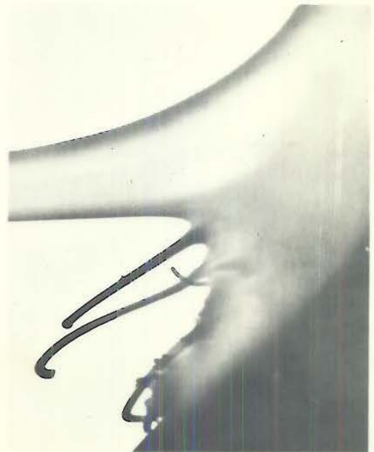
D- RUPTURED POLYSTYRENE RIBBON (20,000X)
