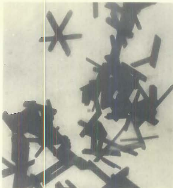
C- LEAD CHROMATE - CRYSTALS AFTER 1 DAY GROWTH (ELECTRON MICROGRAPH-13,000X)
