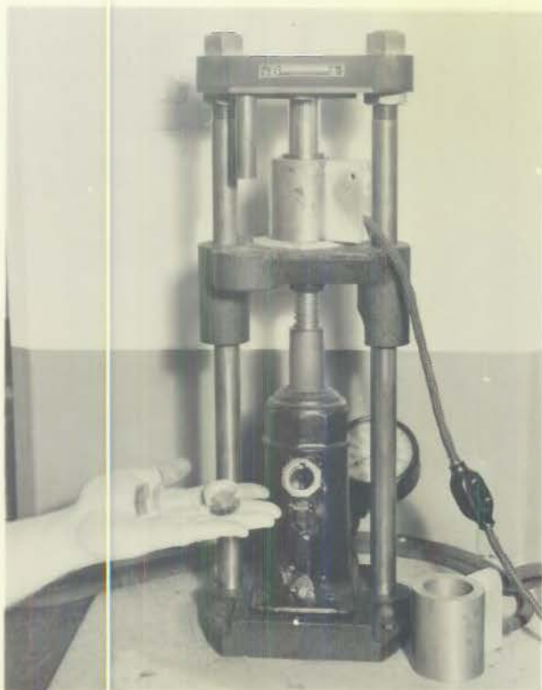
A- PRESS FOR MOLDING METALLIC SPECIMENS IN POLYSTYRENE
