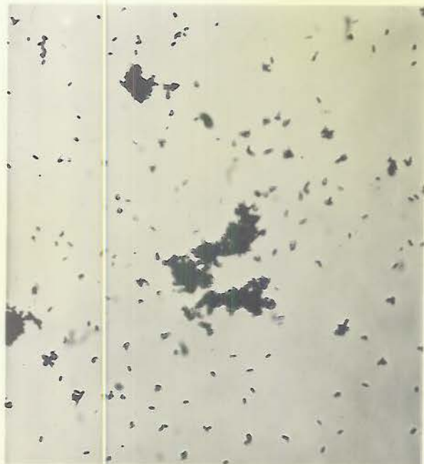
A- LEAD CHROMATE (OPTICAL 675X) CRYSTALS WELL DEVELOPED.
