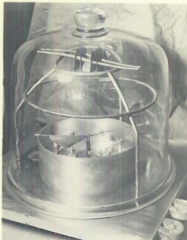
B- EVAPORATION OF SILICA ONTO POLYSTYRENE IMPRESSION
