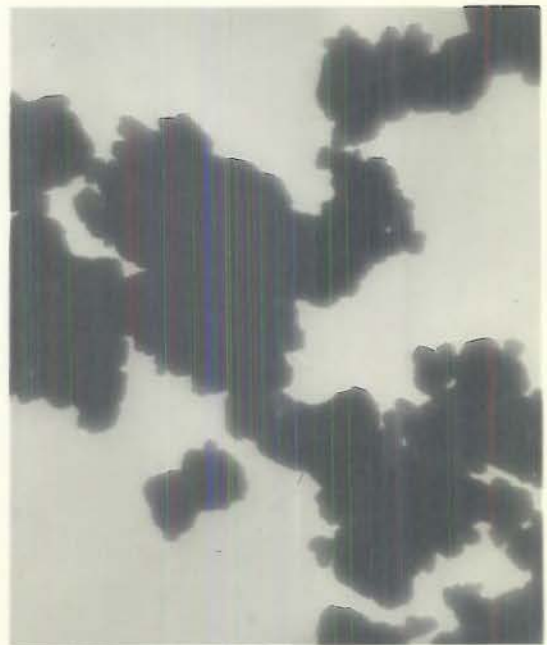
D- ZINC YELLOW (ELECTRON MICROGRAPH 10,000X) PARTICLES DUSTED ONTO BERYLLIUM SUPPORTING FILM
