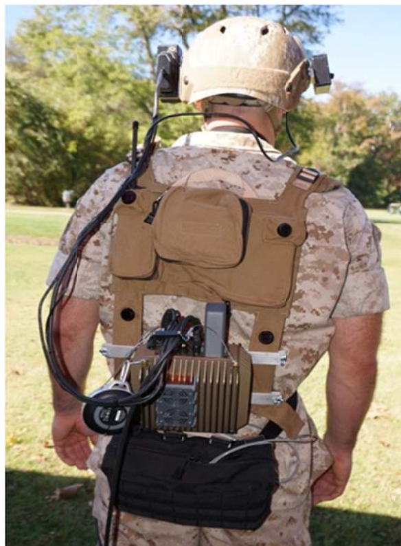
Figure 7: AITT Marine-worn Computer
