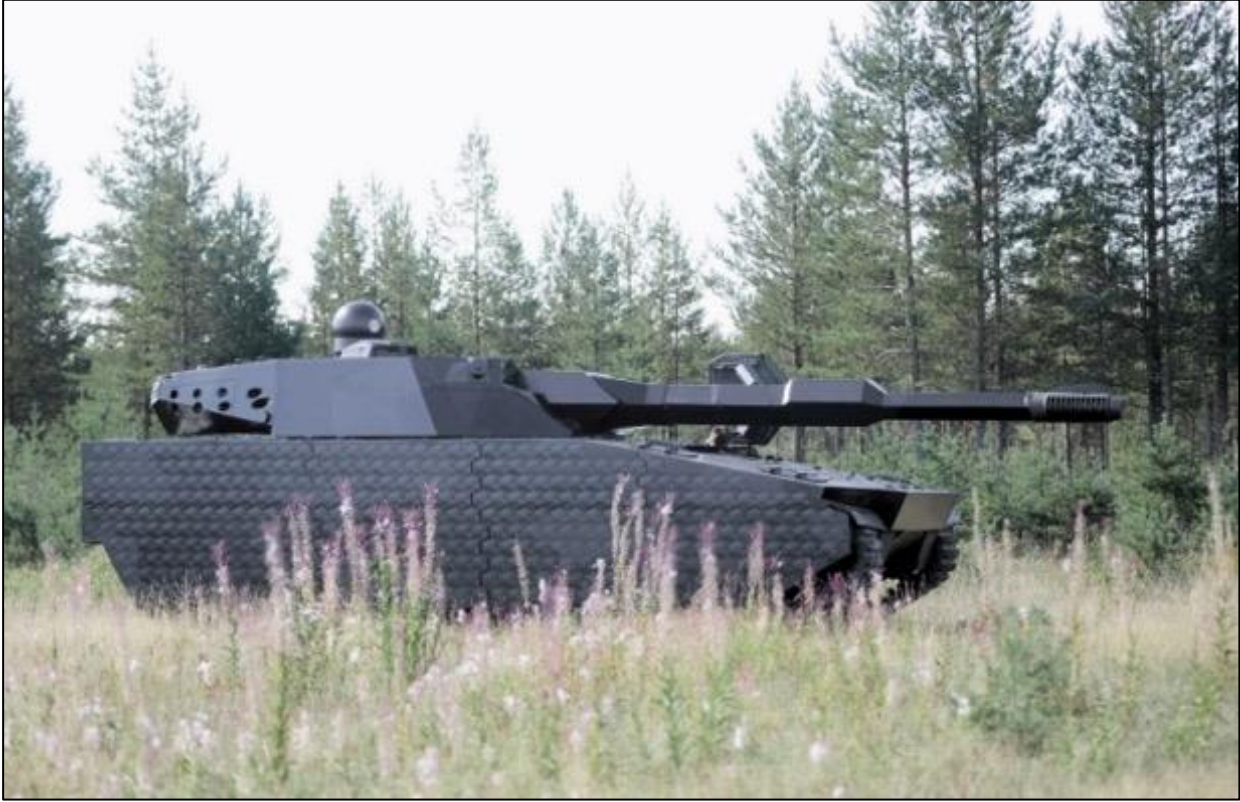
BAE Systems CV 90120-T Technology Demonstrator (off-the-shelf) Armament: 120 mm Main Gun Weight: 35 tons
