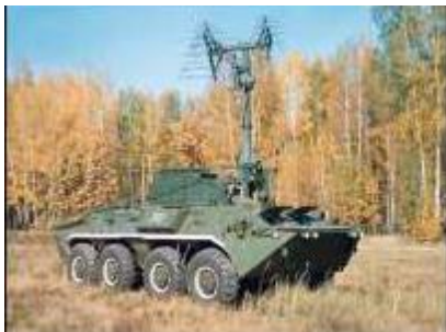
Figure 3: SPR-2 mounted on BTR-80
