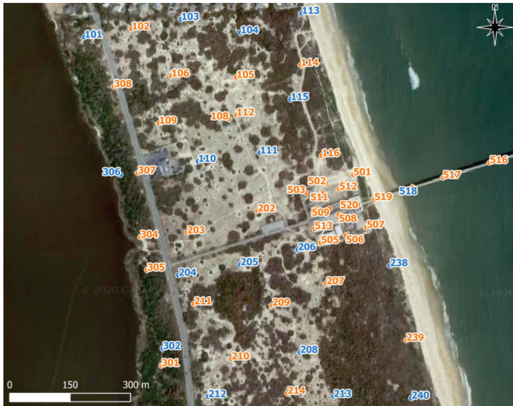
Figure 2-1. GCPs (blue) and checkpoints (orange) across entire FRF property. See Bruder et al. (2018) for more information about ground control point (GCP) distribution.
