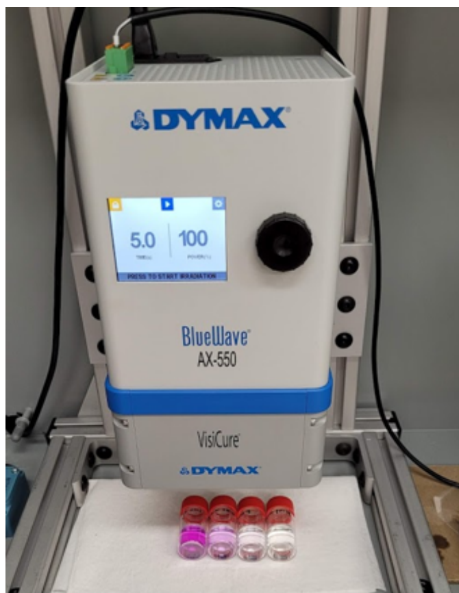
Figure 19: Dymax BlueWave AX-550 VisiCure with four scintillator samples placed in the curing region
