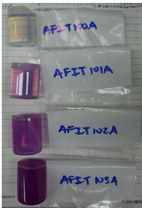
Figure 32: (top to bottom) AFIT 100A (0.01 wt% TPO), AFIT 101A (0.05 wt% TPO), AFIT 102A (0.10 wt% TPO), & AFIT 103A (0.20 wt% TPO) immediately after curing
