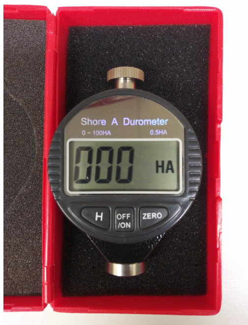
Figure 22: The Shore A durometer employed in this investigation
