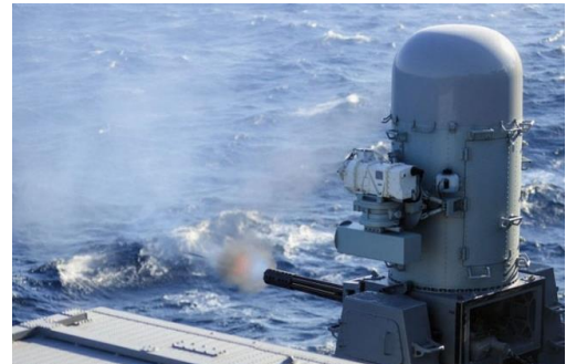
Figure 1. Mk 15 Close-In Weapon System. Weapons: Naval. “Guns. United States,” June 5, 2017, Jane’s Information Group
