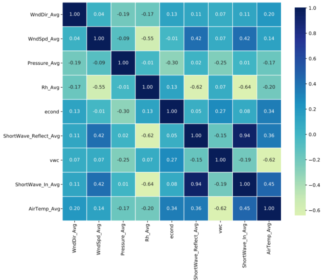
Figure 22. Correlations for CRREL environmental data. Dark blue represents high correlation, whereas yellow denotes poor correlation.
