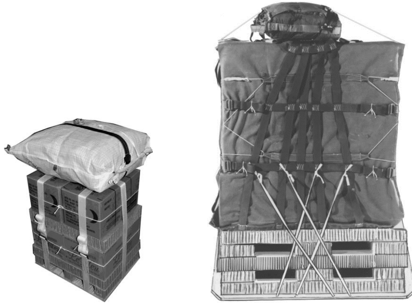
Figure 2: Low-Cost Low-Altitude Bundle vs. Conventional CDS Bundle 67
