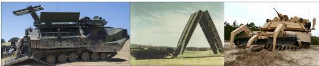
Figure 3: Current mechanized breaching assets, from left to right: Mk154 Mine Clearance Launcher mounted on AAV, an AVLB, and an ABV. Source: Headquarters Marine Corps.
