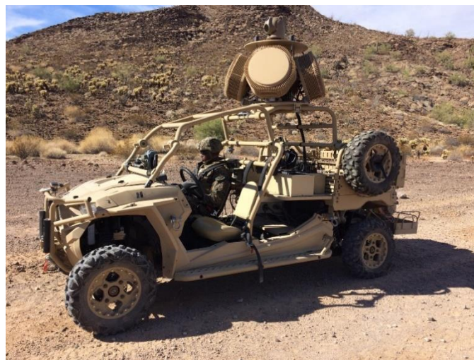
Figure 4. Light Marine Air Defense Integrated System (L-MADIS) integrated into war game to provide on-the-move early warning and cueing against air threats and electronic attack effects.
