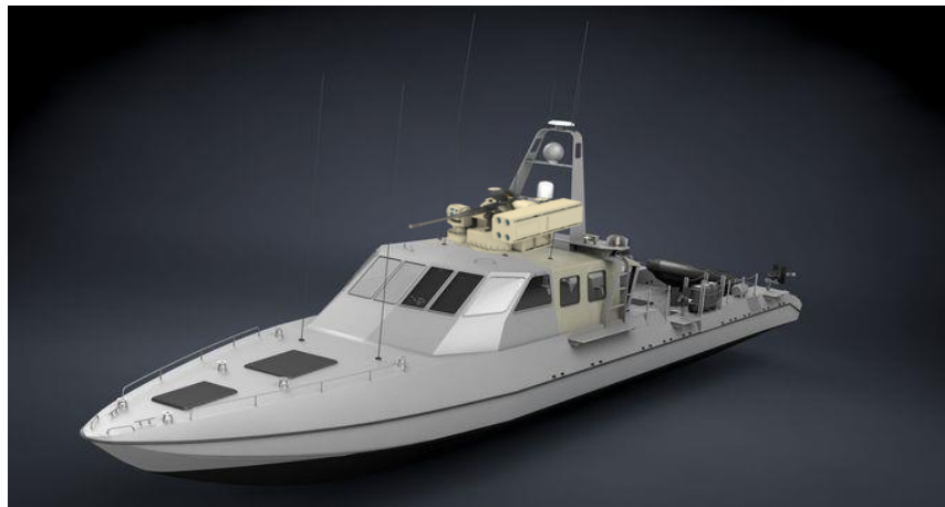
Figure 6. Conceptual Marine Air Defense Integrated System (MADIS) hardware integrated on to the Mark V to provide littoral air defense as an element of a layered defense while augmenting the Maritime Component Commander in sea control operations with the addition of an anti-ship missile.
