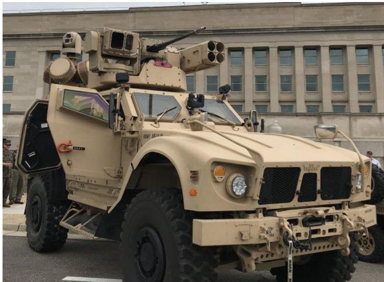
Figure 5. Marine Air Defense Integrated System on display at the Pentagon. The Reconfigurable Integrated Weapons Platform turret currently integrated onto Mine Resistant Armor Protected All-Terrain Vehicle was conceptually integrated on to a Mark V to provide the commander additional flexibility and extended defense in depth during the wargame. 61
