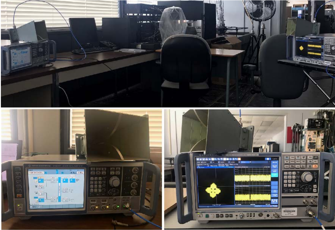
Figure 4.6. Bench OTA testing on pulsed radar embedded communications.
