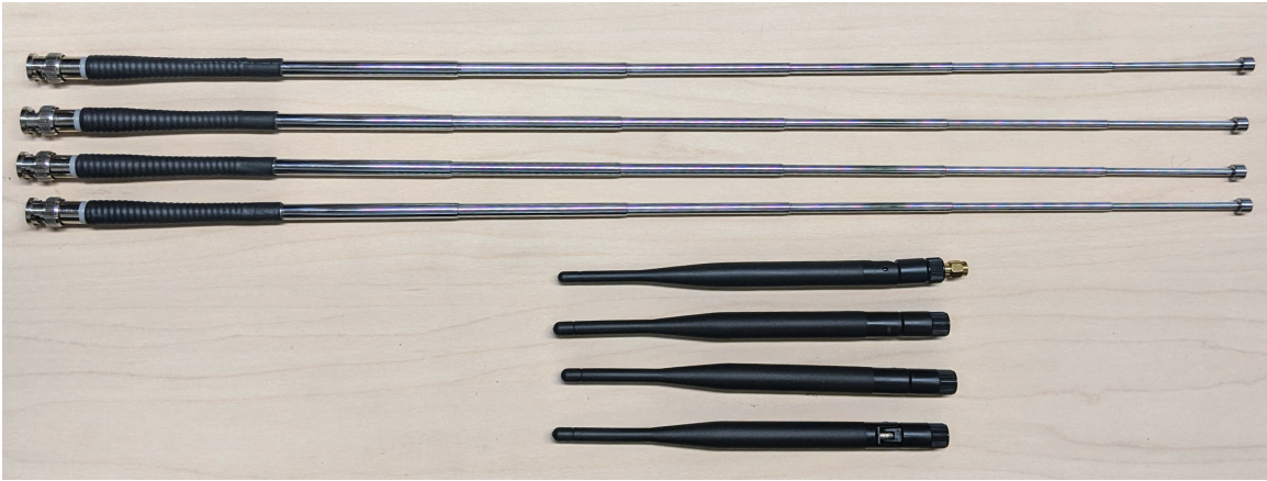
Figure 3.2. Antennas used for testing: 60.2 cm (top), 19.8 cm (bottom).
