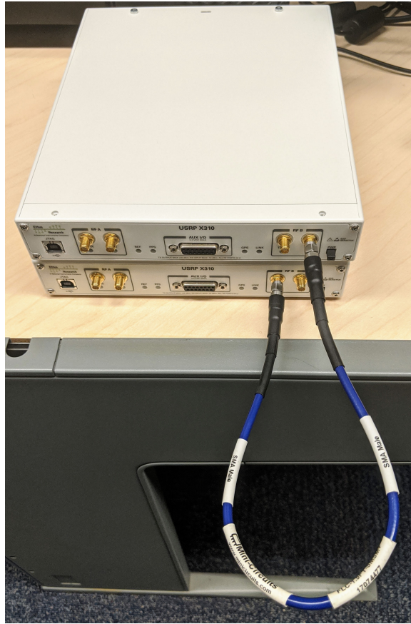
Figure 3.4. SDR-to-SDR baseband configuration.
