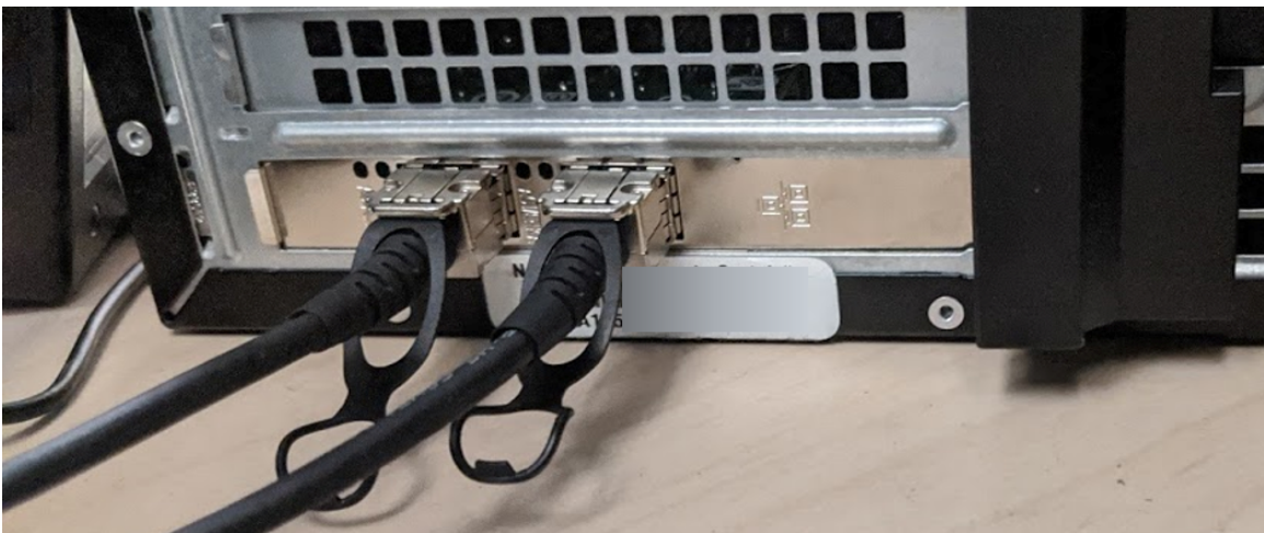
Figure 3.5. Dual NIC to connect two SDRs to one host computer.
