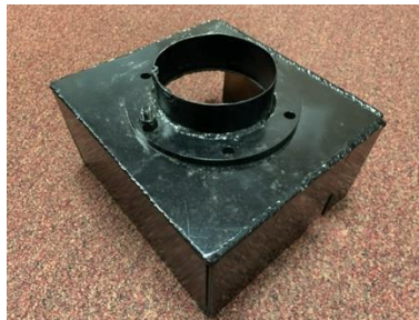
Figure 7. Photo by author of FBCB2/BFT Antenna Cover Fabricated by First Tank Battalion
