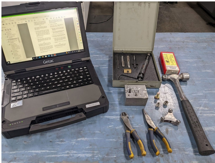
Figure 1. Tools required for “Remove/Install Heli-coil inserts”
