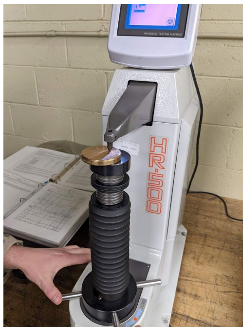
Figure 2. Hardness Tester operation
