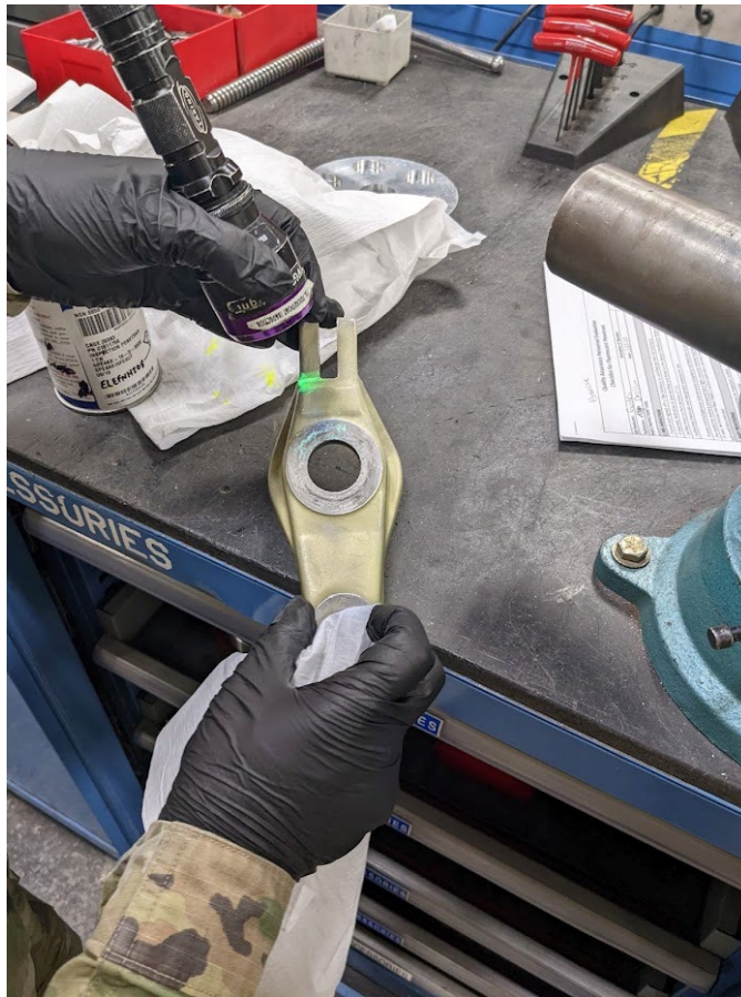
Figure 4. Liquid Penetrant Inspection Method C
