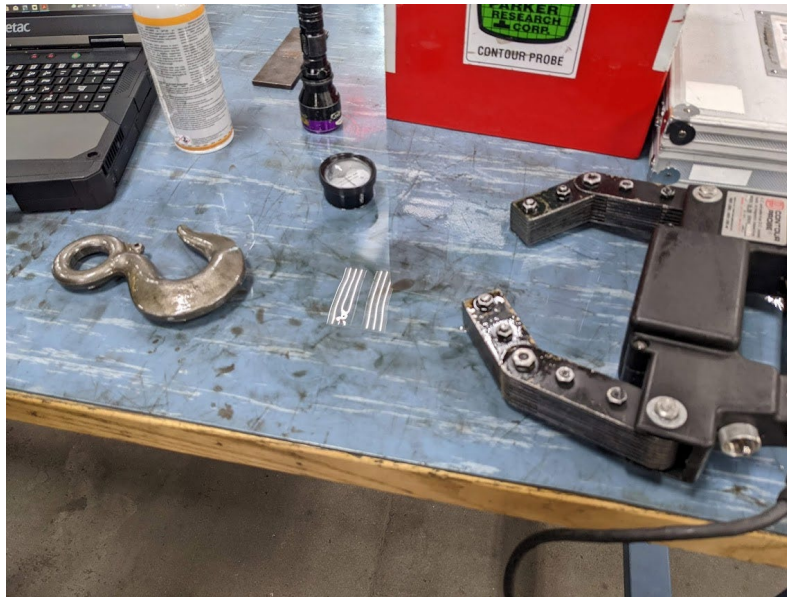
Figure 5. Magnetic Particle Inspection Method
