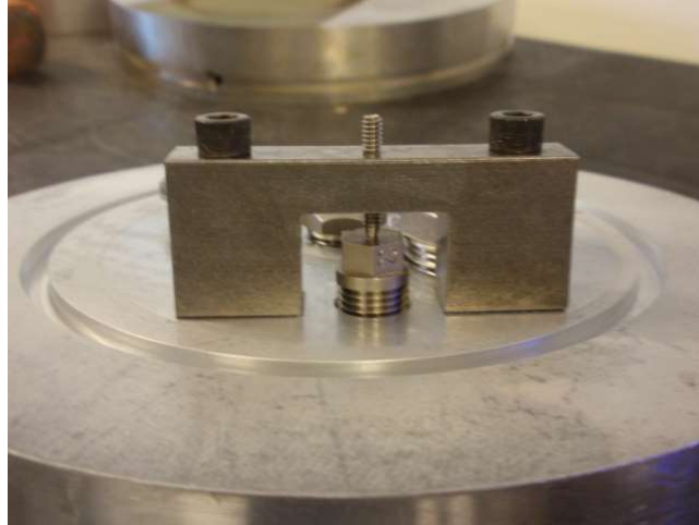
Figure 24: AFM Fixture Mounted Nozzle
