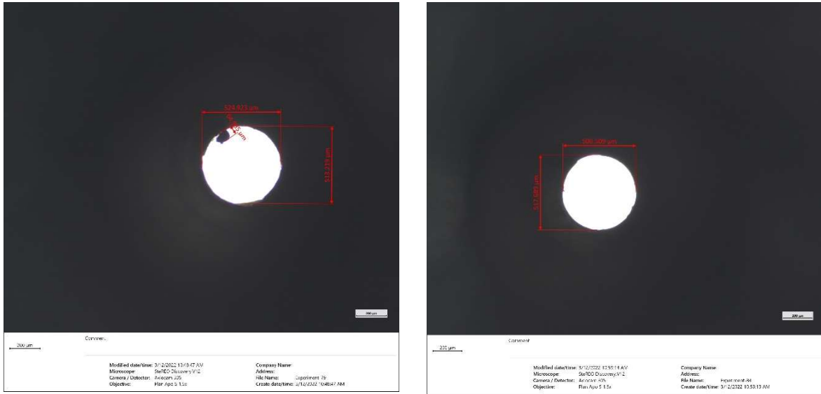
Figure 40: 20-40-1 Milled Protrusion (Left), 20-40-4 Milled (Right)
