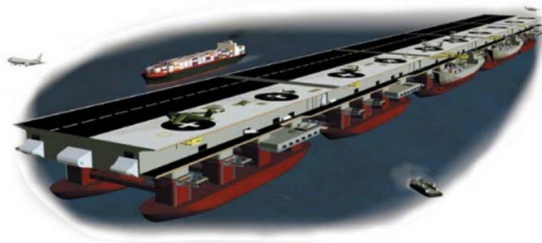
Figure 4. Four individual Joint Mobile Offshore Bases (JMOB) assembled to depict large APOD/SPOD operations and act as a strategically geographic intermediate sea-based supply chain. Image courtesy of Army General Command & Staff College 19
