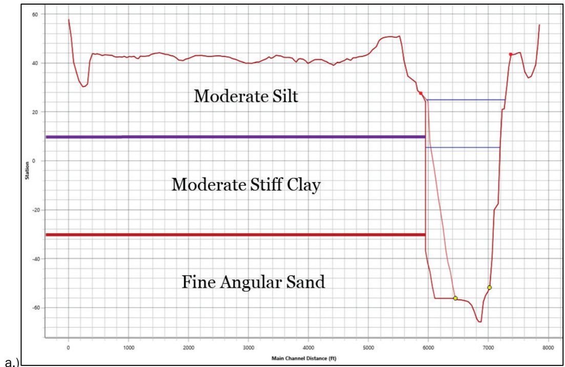
Figure 11. Site 1 cross sections at first and last time-step for parameter sets that yield a.) underestimates and b.) overestimates of bank retreat.
