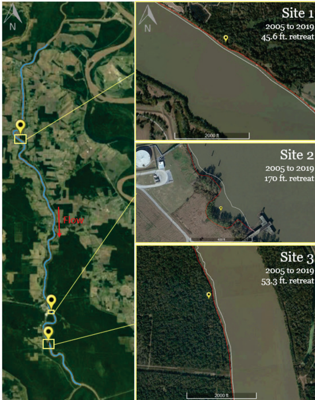
Figure 2. Map showing entire study area with the river centerline (blue) from the HEC-RAS model in the left panel and the three sites initially identified with polylines showing the 2005 (white) and 2019 (red) bank lines, with 2019 imagery as base map, in the right panels.
