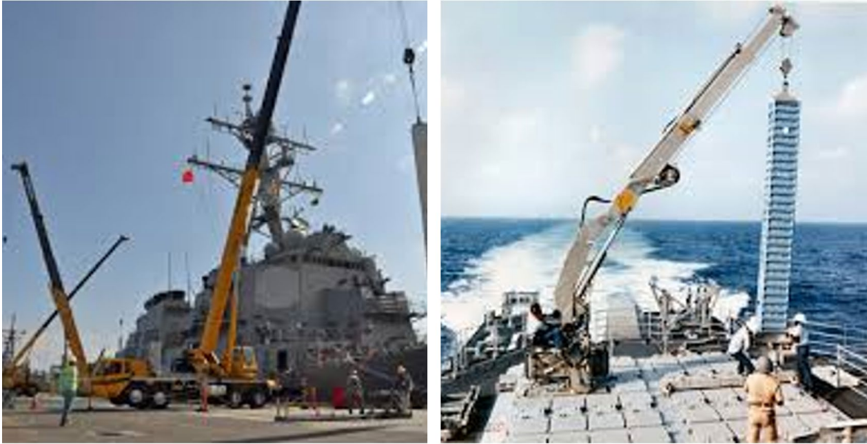
Figure 9: VLS Loading. The left side shows how VLS is currently reloaded in well-developed infrastructure ports. 70 The right shows one at sea VLS reload capabilities being tested. 71
