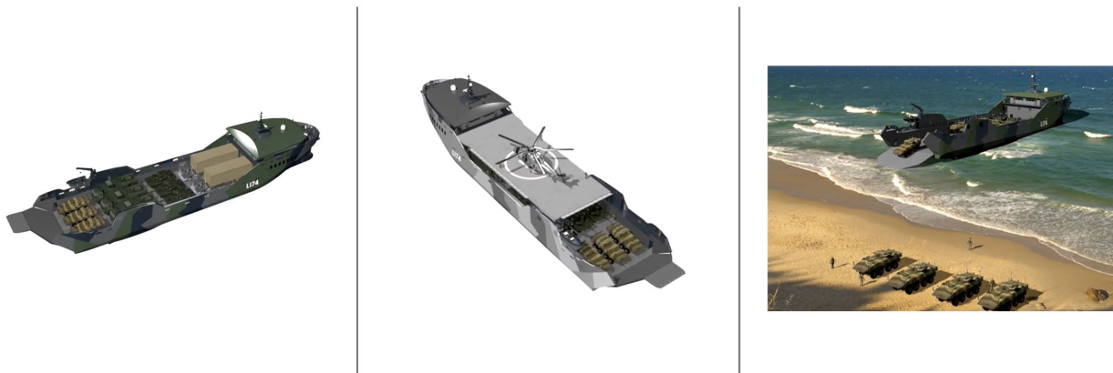
Figure 6: Examples of an OSV, specifically a version called a Stern Landing Vessel (SLV). 52
