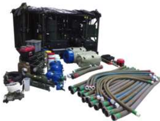
Figure 5. Tactical water purification system (TWPS) Source: "B2605 - Tactical Water Purification System" (Marine Corps Systems Command, n.d.), https://www.marcorssyscom.marines.mil/Portals/105/pdmeps/docs/WATER/B2605.pdf .
