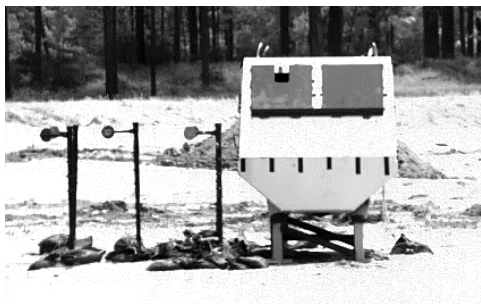
AGH Test Setup for free air detonations (top)
