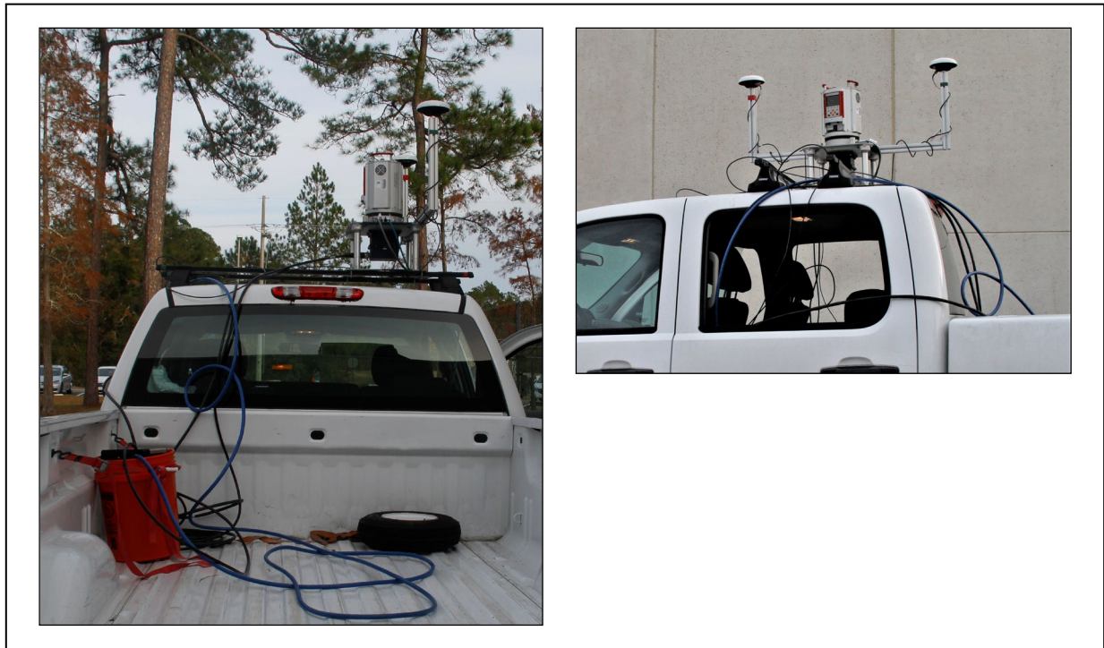
Fig. 3—Proof-of-concept test with single-head MBES, lidar, and IMU (Hode et al. 2019). At left, the MBES transducer head is in an orange bucket secured in the bed of the truck, with the lidar-and-IMU setup secured to a roof rack on the cab of the truck. At right is a side view of the lidar-and-IMU setup on the cab of the truck, with cabling for all of the instruments running through the rear windows.
