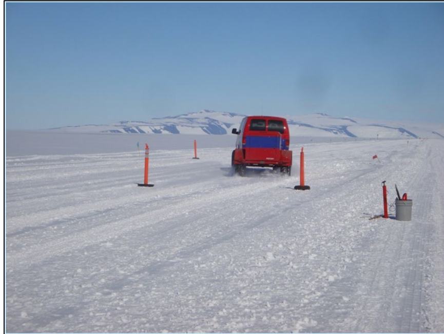
Figure 48. The van and trailer perform a lane-change maneuver to study the vehicle and trailer dynamics, and control, and their impact on the snow-road surface.
