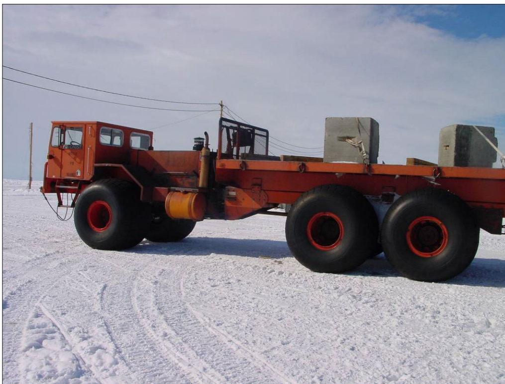
Figure 12. Smooth-tired Canadian Foremost Delta III loaded for compaction.
