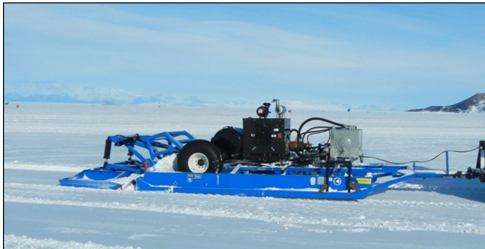
Figure 14. SnowPaver with power-pack upgrade attached, 2012.
