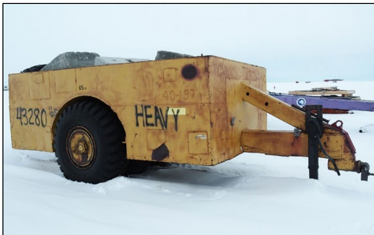
Figure B-9. Heavy ox cart with a 43,200 to 76,200 lb capacity.
