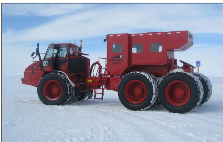
Figure B-10. Kress Articulated Specialized Transport Truck (CAT730) used primarily with cargo or passenger trailers.
