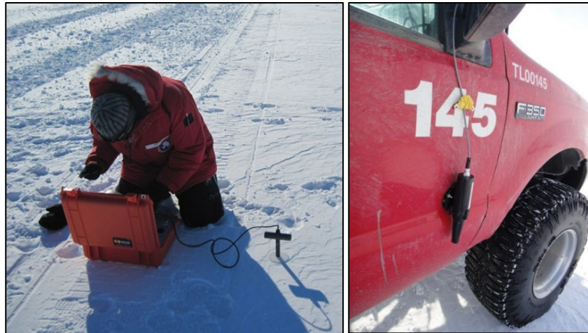
Figure 21. Temperature measurements using a thermocouple probe at each monitoring location along the roads ( left ) and an infrared sensor mounted on a vehicle and driven along the snow roads ( right ).
