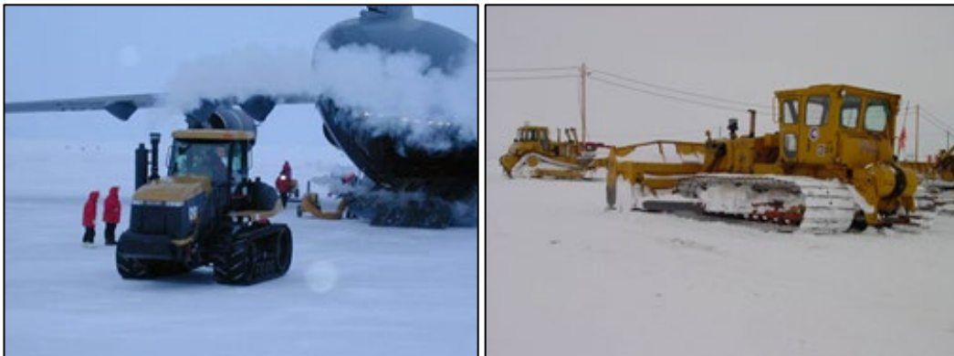
Figure 8. Caterpillar Challenger 95E ( left ) and Caterpillar low ground pressure (LGP) “stretch” D8 ( right ).
