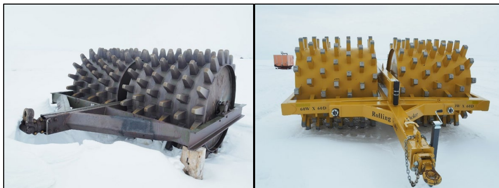
Figure B-8. Sheepfoot compactors.
