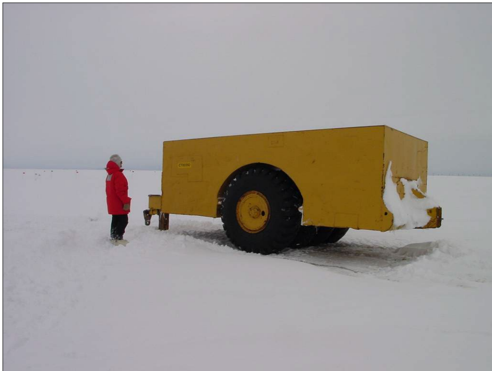
Figure 11. The 34,400–67,400 lb capacity pneumatic-tire load cart.
